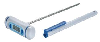
This compact thermometer measures temperature over the range of -49.9 to +149.9 °C. The thermometer features a  $\emptyset 3.5 \times 120$ mm pointed stainless steel probe. The instrument incorporates a °C/°F switch and a display hold feature. Each unit is supplied with a probe cover that incorporates a pocket clip.
