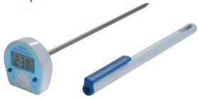
This dial-shaped thermometer measures temperature over the range of -49.9 to  $+149.9^{\circ}$ C. The thermometer features a Ø3.5 x 125mm pointed stainless steel probe. The instrument incorporates a °C/°F switch and a display hold feature. Each unit is supplied with a probe cover that incorporates a pocket clip.
