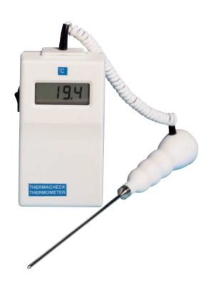
The ThermaCheck thermometer is supplied complete with a permanently attached, general purpose, food penetration probe with a 130mm stainless steel stem and a one metre coiled PU lead.
