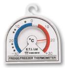
This fridge or freezer thermometer has a  $\varnothing 70$ mm dial, indicating temperature over a range of -30 to +30°C in 1°C divisions and incorporates colour-coded zones. The ABS case measures 70 x 60mm. The thermometer can be free-standing or hung from a shelf.
