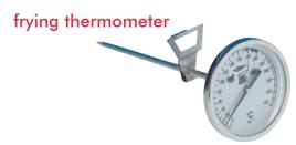
The frying thermometer incorporates a  $\varnothing 50$ mm dial and a pointed, stainless steel  $\varnothing 4$  x 150mm stem. The frying thermometer indicates temperature over the range of 0 to  $+300^{\circ}$ C in  $10^{\circ}$ C divisions. For the most accurate temperature recording, insert the thermometer in the thickest part of the product. The dial is clearly marked for meat, poultry, fish and chips.
