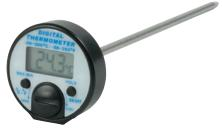
This dial-shaped thermometer measures temperature over the range of -49.9 to  $+199.9^{\circ}$ C. The thermometer features a Ø3.5 x 120mm pointed stainless steel probe. The instrument incorporates a max/min memory function, a display hold feature and is °C/°F switchable. Each unit is supplied with a probe cover and pocket clip.
