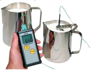
These stainless steel probe holders, clip on the top of a jug or similar to hold in place a temperature probe. Two models are available, one that will accept either a Ø3mm or Ø3.3mm probe stem and the other is designed to work in conjunction with a bi-metal thermometer and will accept a Ø4mm probe stem. The probe should not touch the bottom or the sides of the container.
