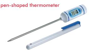
This compact thermometer measures temperature over the range of -49.9 to +149.9 °C. The thermometer features a  $\emptyset 3.5 \times 120$ mm pointed stainless steel probe. The instrument incorporates a °C/°F switch and a display hold feature. Each unit is supplied with a probe cover that incorporates a pocket clip.
